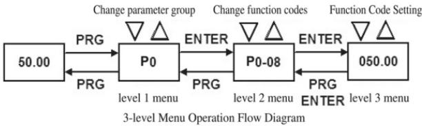
Description: Under the level 3 menu, user can press PRG or ENTER to back to the level 2 menu. The difference is that by pressing ENTER, it saves the setting parameter before getting back to the level 2 menu and then it enters the next function code automatically; by pressing PRG, it will directly return to the level 2 menu without saving parameters.
