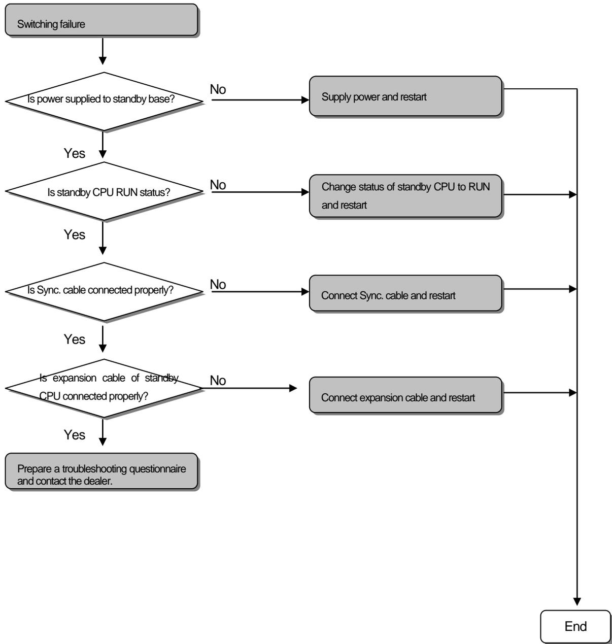
15.2.11 When expansion cable is disconnected
