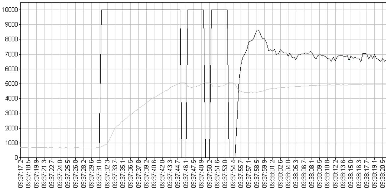
The above graph is the water level waveform gained by setting `_PID[B]_[L]HYS_val` value (50 in the example) properly and MV should have 3 square waveforms as seen in the figure.
