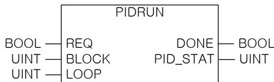
If inputting block number (0 ~ 7) into BLOCK and loop number (0 ~ 31) into LOOP, a loop of the block is selected. PID\_STAT displays the operation information for a PID loop, `_PID[B]_[L]STATE`.
