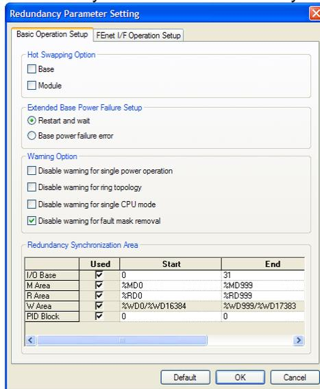
Different from other parameters, the redundancy parameters can be written during running.
