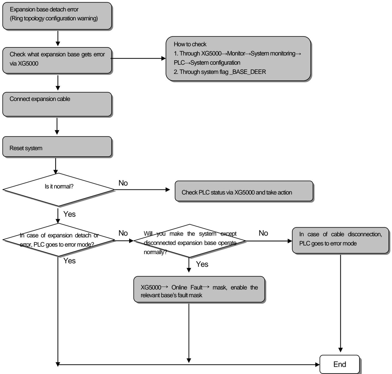
(2) system except detached expansion base operates normally: in case of enabling fault mask
