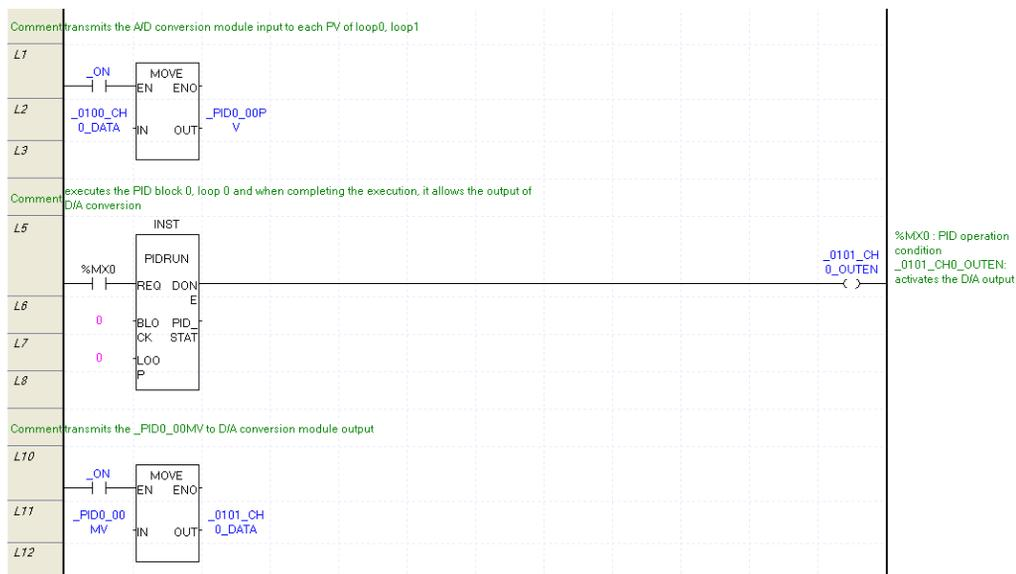
L1 : delivers Analog input data to PV of PIDRUN instruction by using constant On contact.
