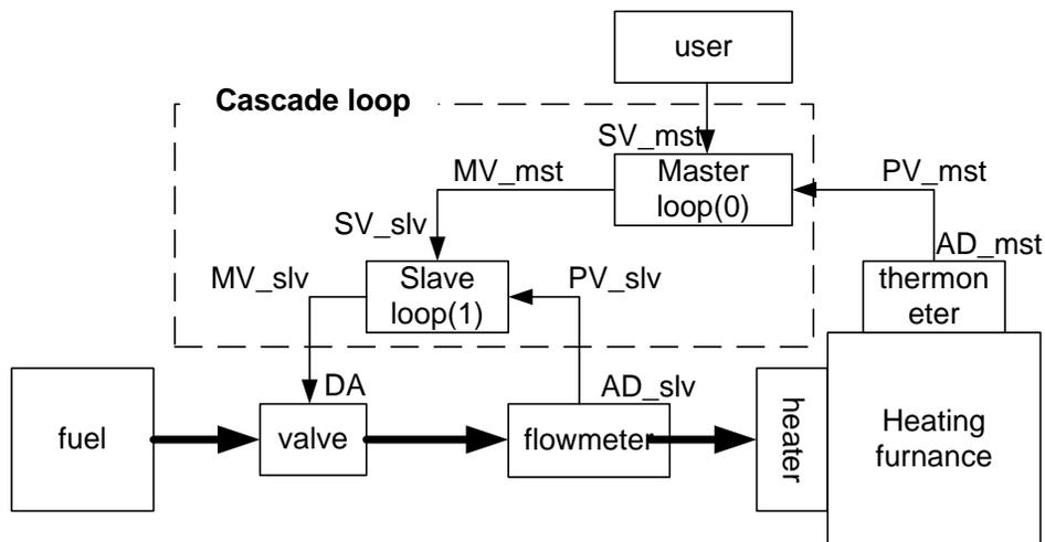
The above block diagram is the system to measure the temperature of heating furnace, supply fuel to the heater and maintain a desirable temperature.
