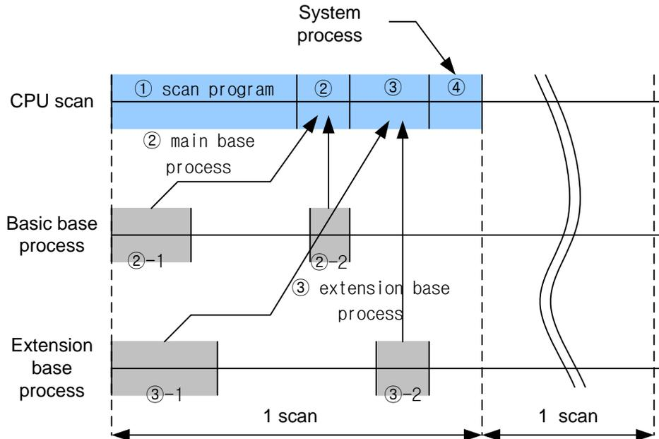
Scan time = ① scan program process + ② basic base process + ③ expansion base process + ④ system process
