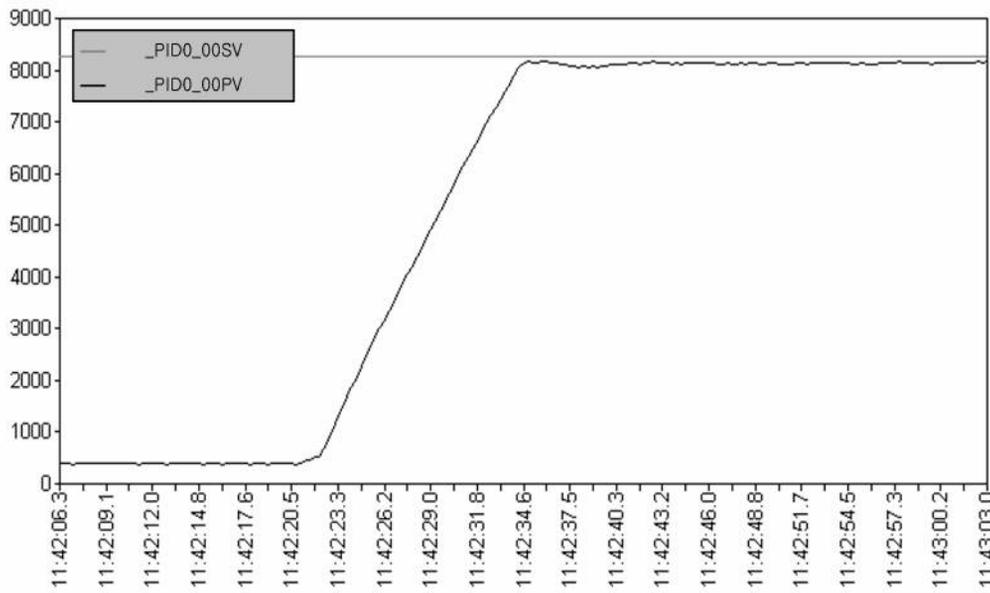
Due to too large T<sub>i</sub>, the normal state residual drift lasts and there is a slight overshoot.
