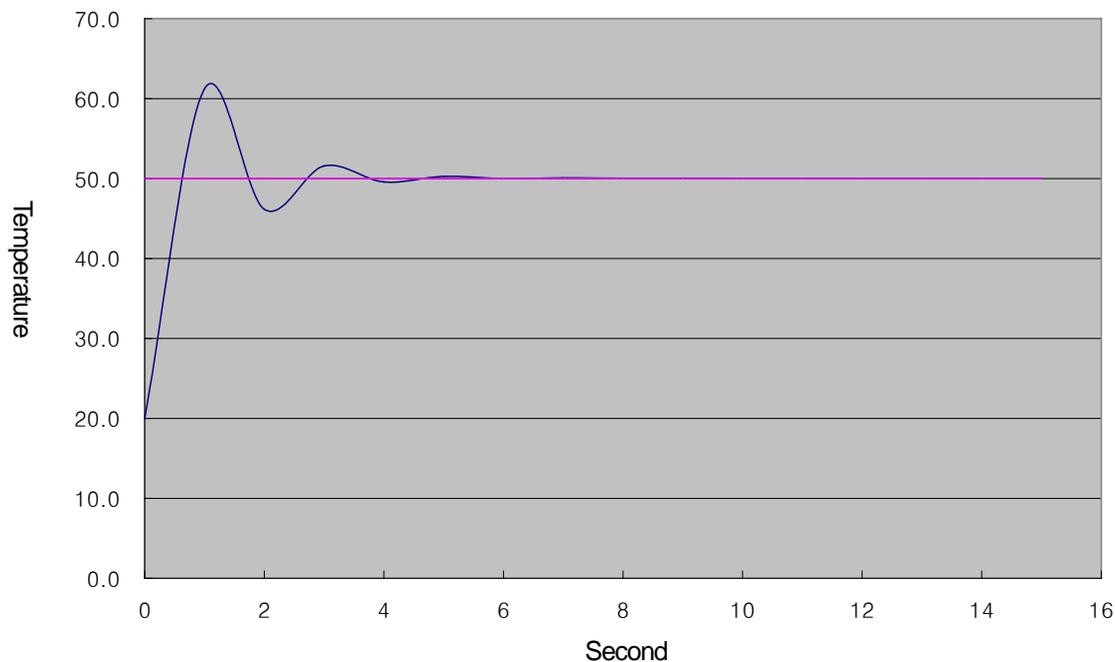
As a result of adding integral effect, the residual drift disappears and the system is converged to 50°C accurately. However, the temperature temporarily increased more than a desirable temperature, for which it increased up to 61.2°C and dropped, deepening overshoot. Excessive overshoot may overburden the system or make it unstably, so it is necessary to relieve the overshoot through proper coefficient tuning or improve it by means of PID control applying differential effect.
