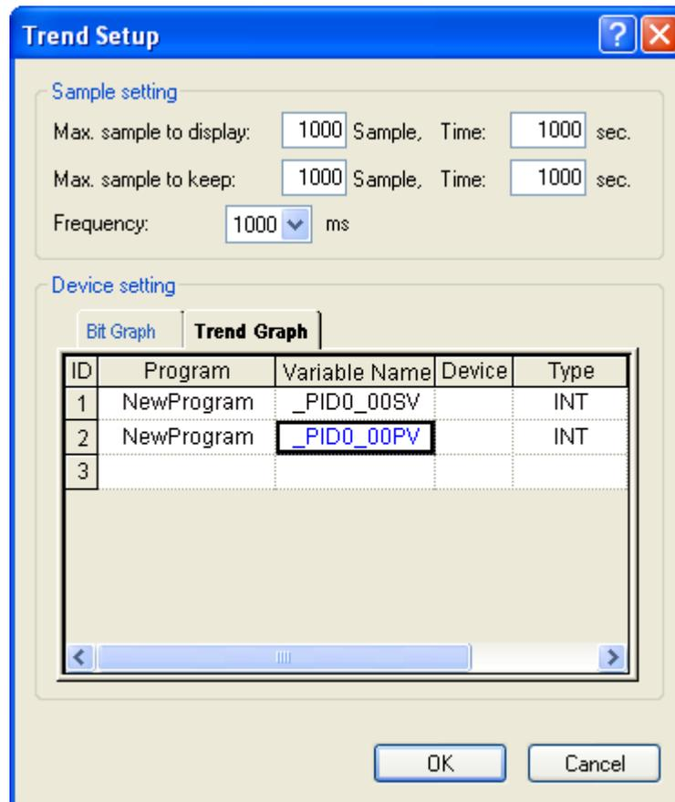
Set the monitoring cycle as 200ms, select the trend graph tab on the bottom and register the parameters to monitor such as SV and PV of block 0 and loop 0.
