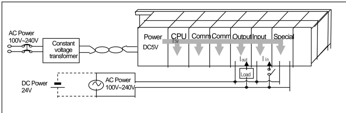
[Figure 8.4.1] Example of use of power module
