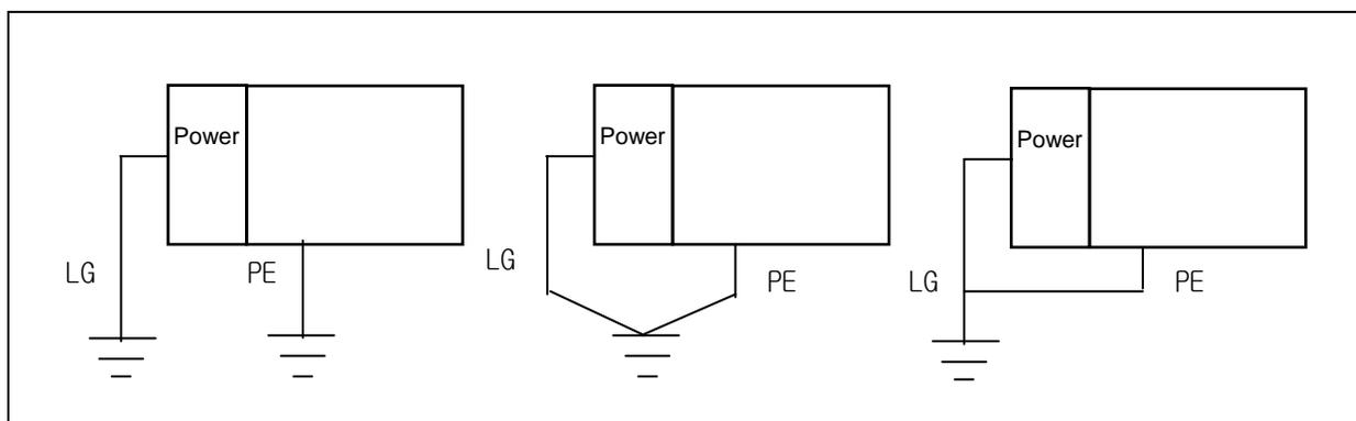
A) Exclusive grounding : best    B) common grounding : good    C) common grounding: defective
