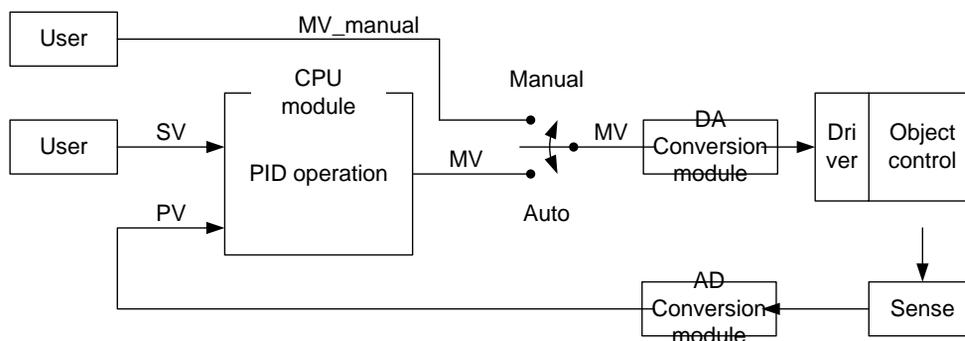
As presented in the above figure, PLC functions as a control in a whole control system while sensor and driver are used to detect an object to control and drive the system, respectively.
