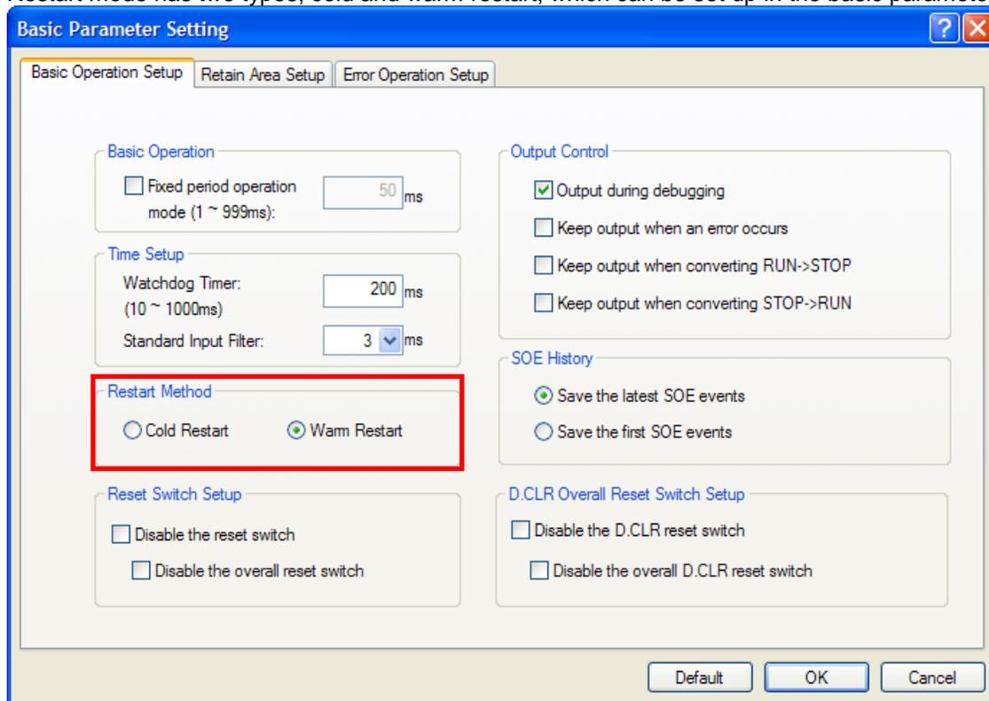
When the standby CPU starts up, it executes the initialization according to the restart mode and receives the program and data backup from the master. When set up in flash operation mode, it receives the flash data backup from the master too.
