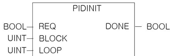
If inputting block number (0 ~ 7) into BLOCK and loop number (0 ~ 31) into LOOP, a loop of the block is selected.
