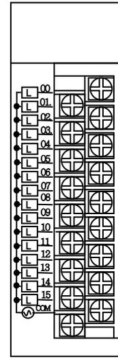
9.3.5 16 point transistor output module (sink type)
