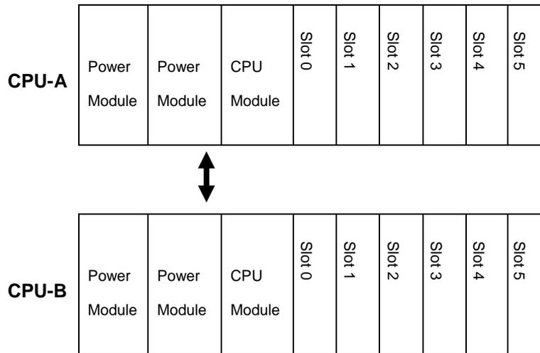
[Fig. 2.3.2] Slot configuration of duplicated basic base
