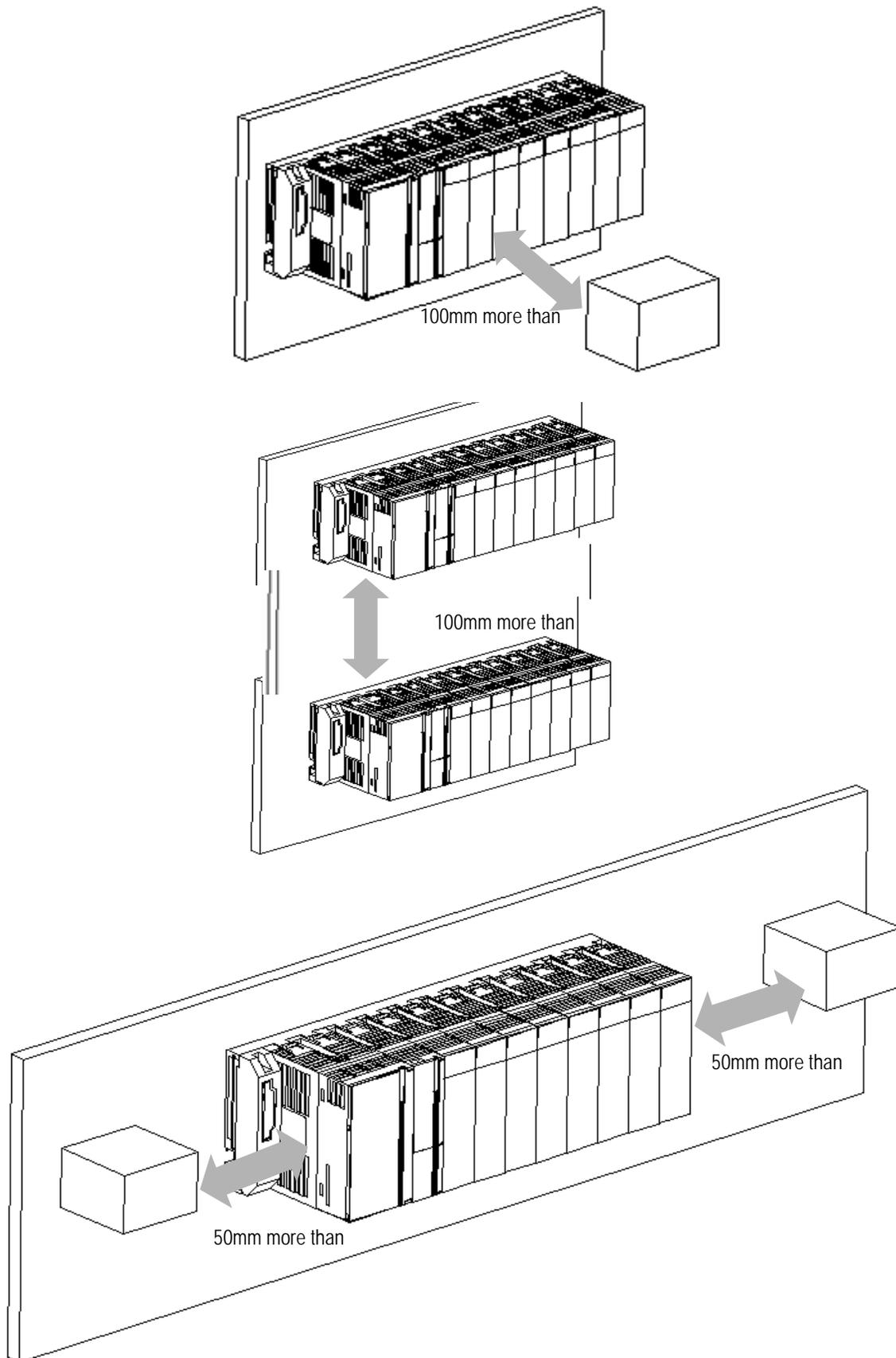
(h) In a layered-installation of PLCs, the temperature of the base at the top may become very high due to the heat transferred from the lower layers. If the temperature in the control cabinet is high, install a ventilating fan, or provide sufficient distances between the bases.
