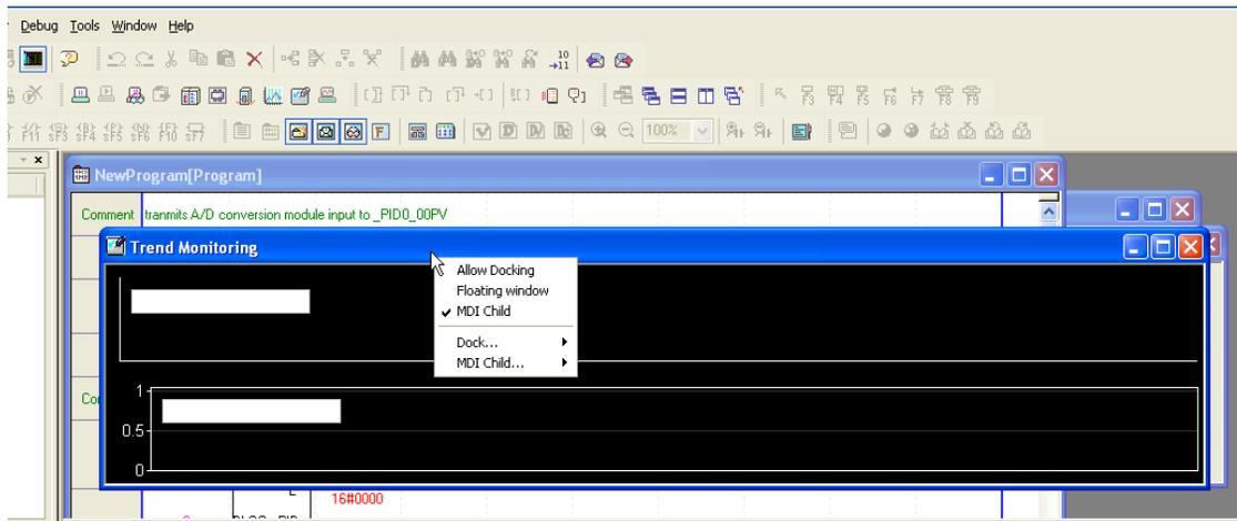
By allowing the docking of trend monitor, arrange it properly.
