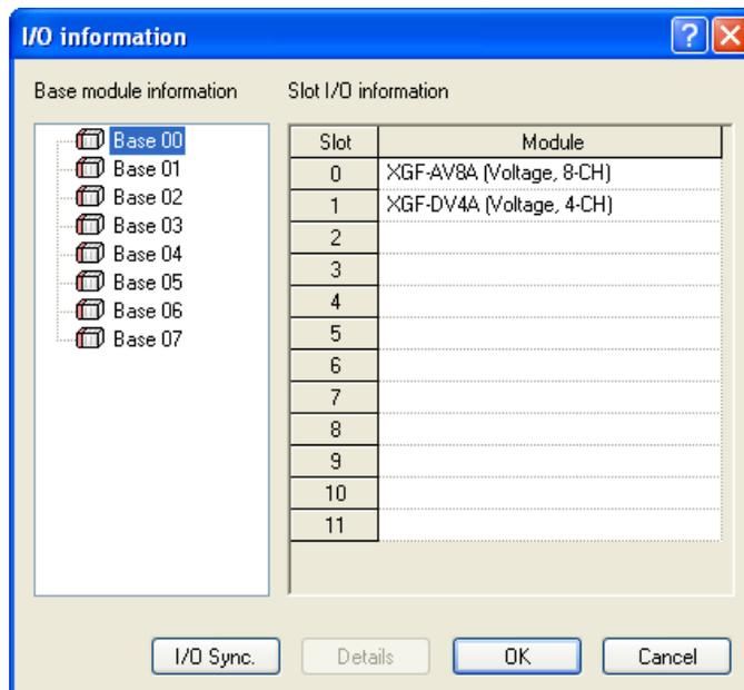
Once a module is registered, it is necessary to register a parameter to use among the parameters assigned to the module, as the global parameter.
