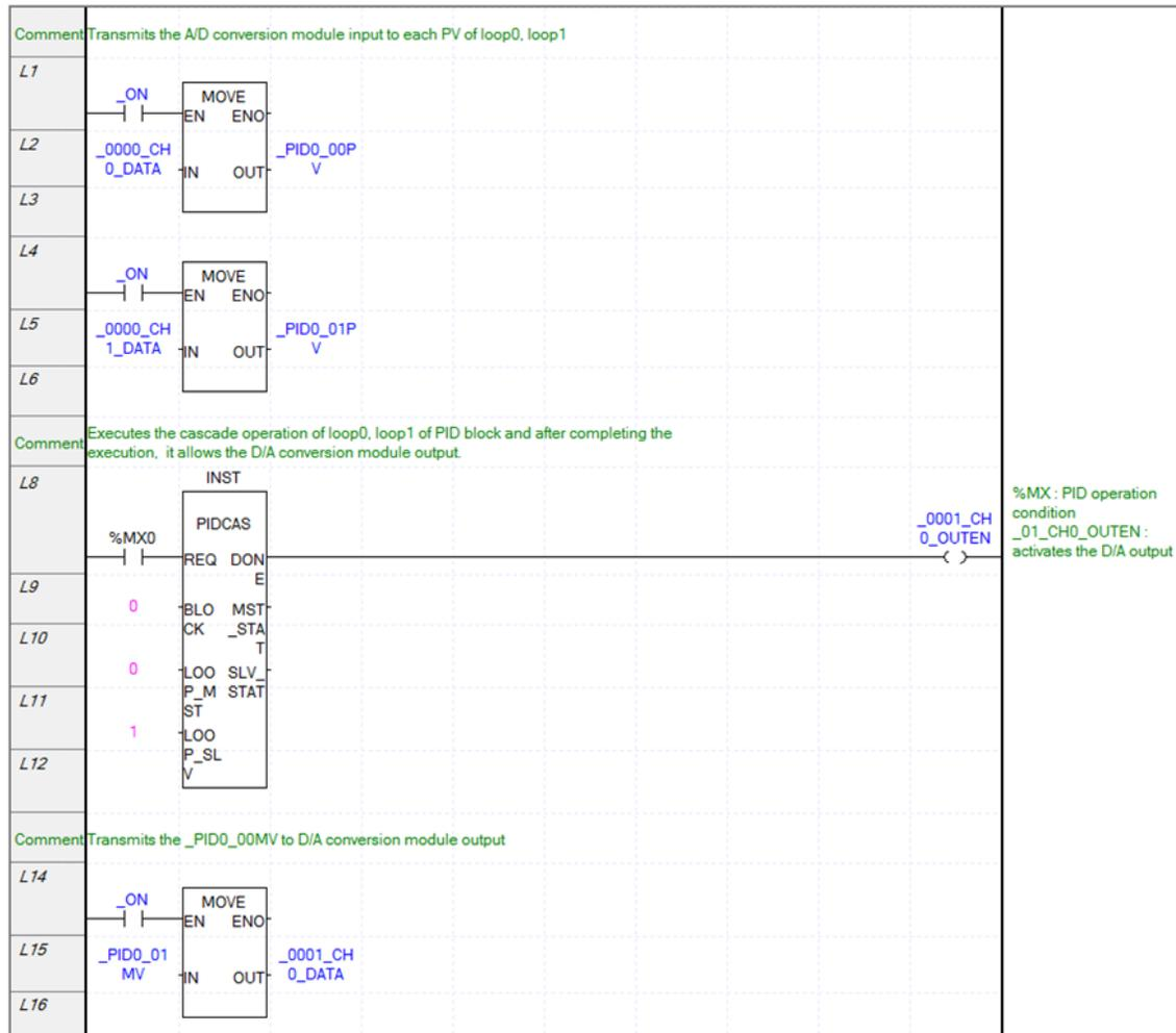
The above ladder program is the view of cascade configuration, based on the following block diagram.
