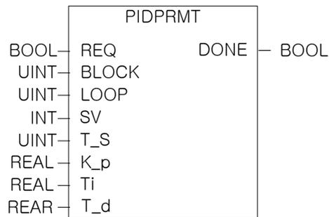
If inputting block number (0 ~ 7) into BLOCK and loop number (0 ~ 31) into LOOP, a loop of the block is selected.
