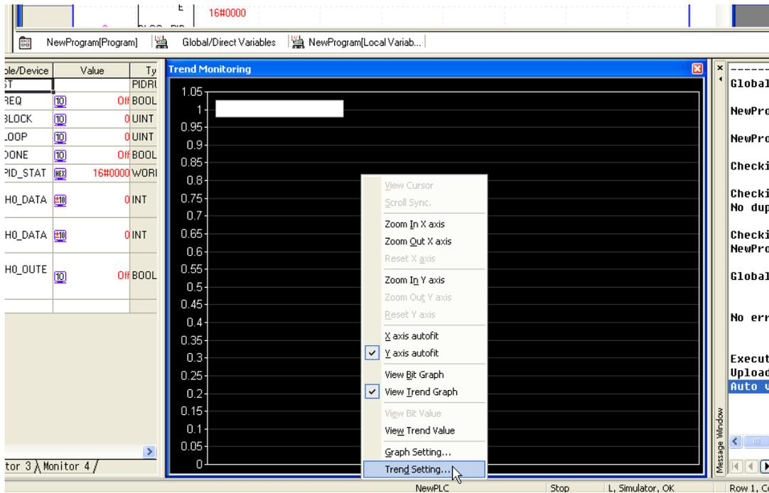
By means of trend setting, register the data to observe.
