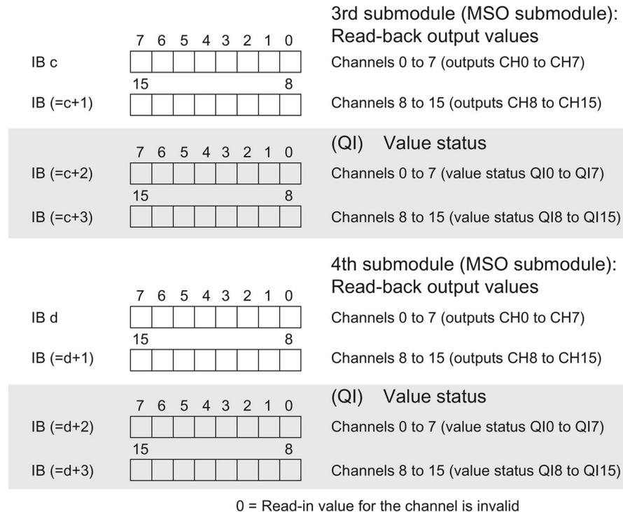
Figure 4-4 Address space for configuration as 1 x 16-channel DQ 16x24VDC/0.5A ST S MSO with value status
