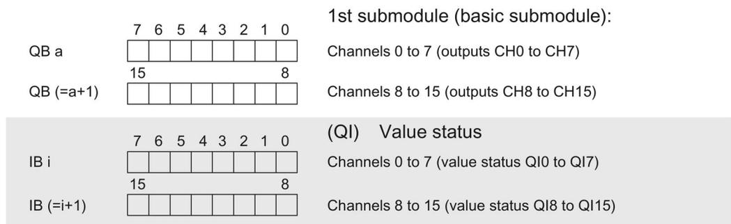
Assignment in the process image input (PII) for 2nd submodule
