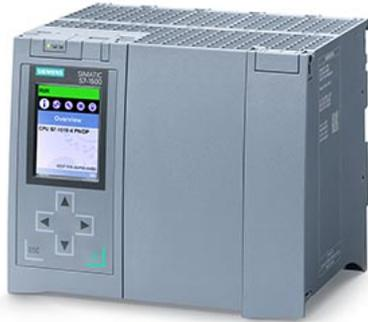
SIMATIC S7-1500, CPU 1518-4 PN/DP, Central processing unit with work memory 4 MB for program and 20 MB for data, 1st interface: PROFINET IRT with 2-port switch, 2nd interface: PROFINET RT, 3rd interface: Ethernet, 4th interface: PROFIBUS, 1 ns bit-performance, SIMATIC Memory Card required
