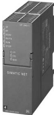
Communications processor CP 343-1 for connection of SIMATIC S7-300 to Industrial Ethernet via ISO and TCP/IP, PROFINET IO controller or PROFINET IO device, integrated 2-port switch ERTEC 200, S7 communication, fetch/write, send/receive with and without RFC1006, Multicast DHCP, NTC- CPU Sync, diagnostic, initialization via LAN, 2x RJ45 connection for LAN with 10/100 Mbit/s
