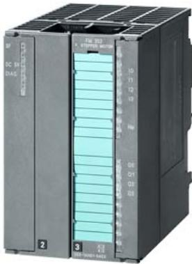
SIMATIC S7-300, FUNCTION MODULE FM 353, FOR POSITIONING
